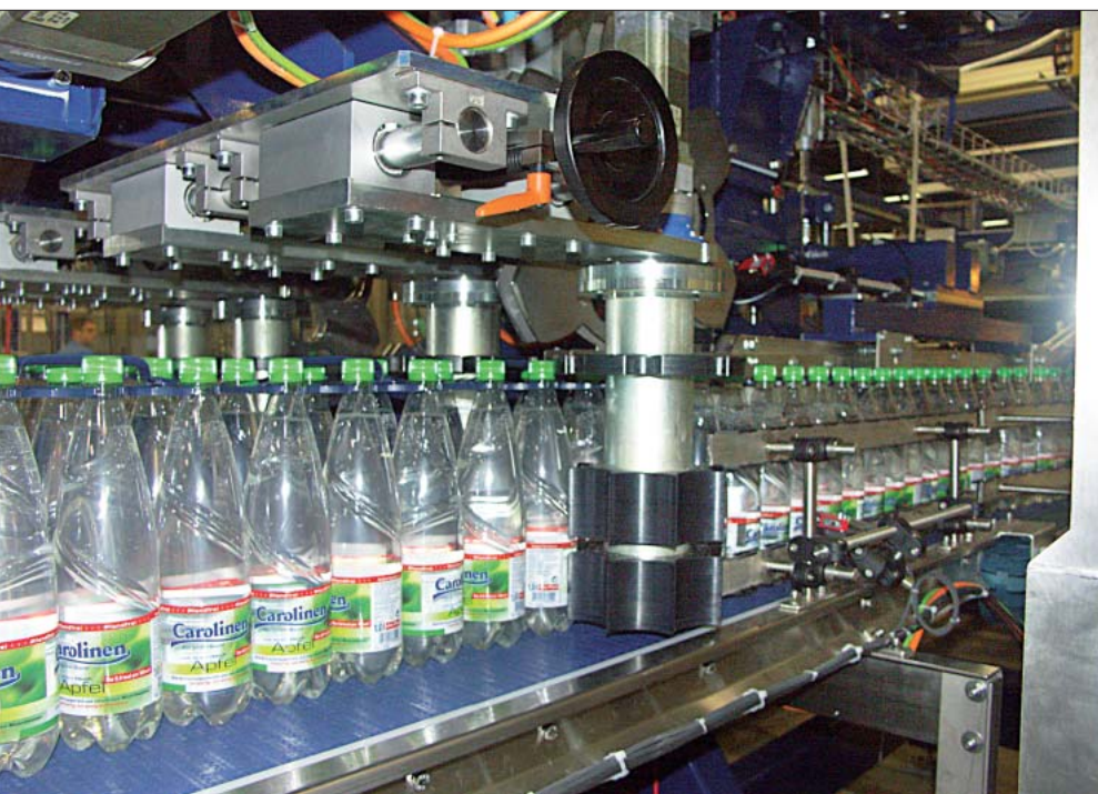
The Carriers are supplied from above and the bottles are pressed into the holds in a merging lane system by means of star-shaped wheels.
